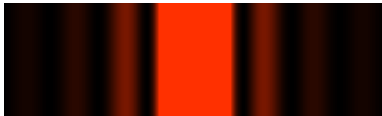
Interference pattern for light with a wavelength of 633 nm behind a single slit
